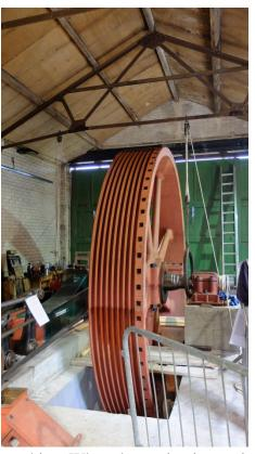
Tony N has rigged up a natty little gadget on the second motion fly-wheel oil aquariums of the Roberts engine. Unless one climbs up to them, it is difficult to see if the oil is running into the bearings. Tony has placed three small battery operated LED lights in the oil reservoirs. They can easily be seen from the back of the engine, and the ones which are immersed in oil appear orange but if any appear white, it means they are out of the oil and the level is dropping. Well done, that man.
