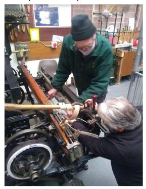
mechanism is missing some metal parts which can be fairly easily made, but we also need a complete set of Dobby Lags, which are the wooden bars with holes and pegs which control the healds in a similar way to the cards in a Jacquard Loom.
