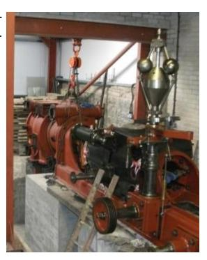
made to get on with it. The casting will have to be machined now and attention given to a cracked piston ring, but things are going on, and the momentum is being maintained.
