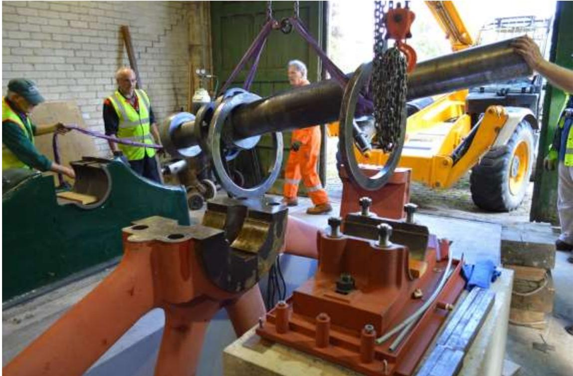
**Figure 3: The main shaft is brought into place**
