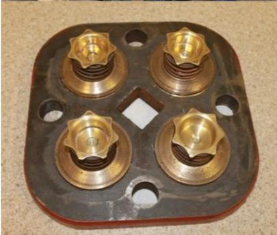
The Boiler feed pump (bottom) for the Cornish boiler had surgery during last year to replace a valve block, that block has been rebuilt following the discovery that four parts had been missing from it right from its arrival at Bancroft. The valve assembly was on display until the end of 2013 in the Engine Hall. A complete strip and overhaul of the spare pump that we hold is to start very shortly and it is hoped that it will be on display whilst the work proceeds.
