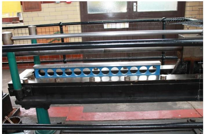
when checked with a high precision box level was co-planar within 0.002"/36" of the crosshead slideway. With the 1910's equipment available to William Roberts for manufacture, the kind of kit for installation and after 90 years of work, these are amazing results
