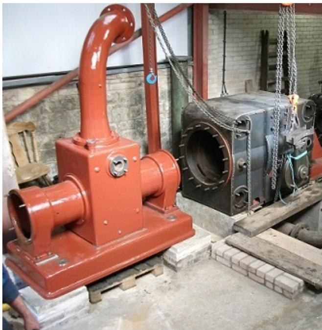
*Some more work has been done to the Bradley Engine. John R. and Ian A. have been working on the air-pump and condenser. It has been cleaned and painted, and placed in position at the rear of the engine, and more pipe-work added. It rests on brick piers built by Roy F.*
