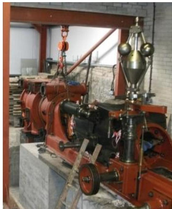
*made to get on with it. The casting will have to be machined now and attention given to a cracked piston ring, but things are going on, and the momentum is being maintained.*
