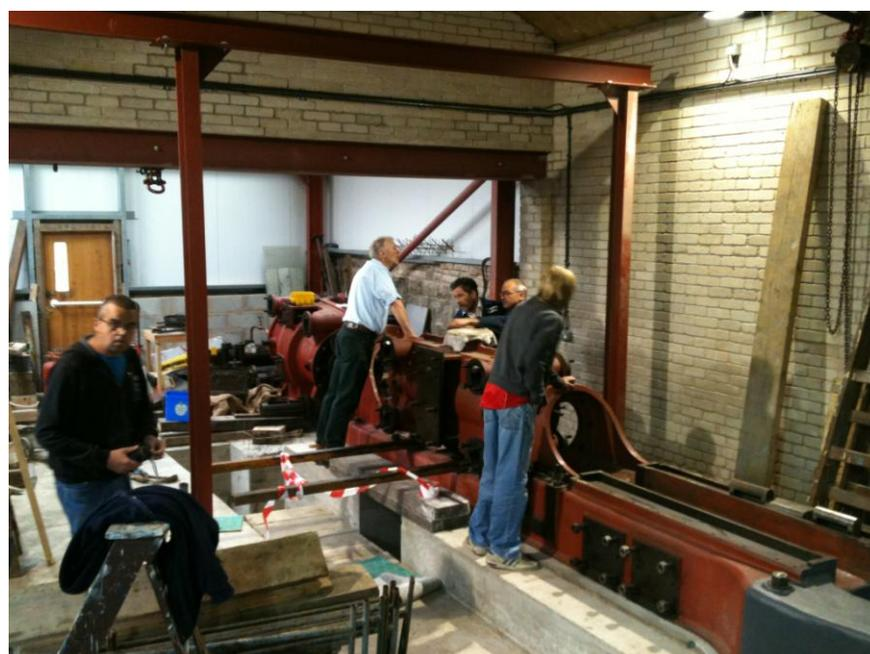
It's not all doom and gloom, however. The high-pressure cylinder is now in position on the engine bed, and whilst we decide how to sort out the piston problems, there is nothing to prevent us from assembling the valves and valve gear on the high-pressure cylinder, and mounting the governor in position. If we do that, it will certainly look more like an engine. There are quite a few visitors who come regularly, and I always think they must
