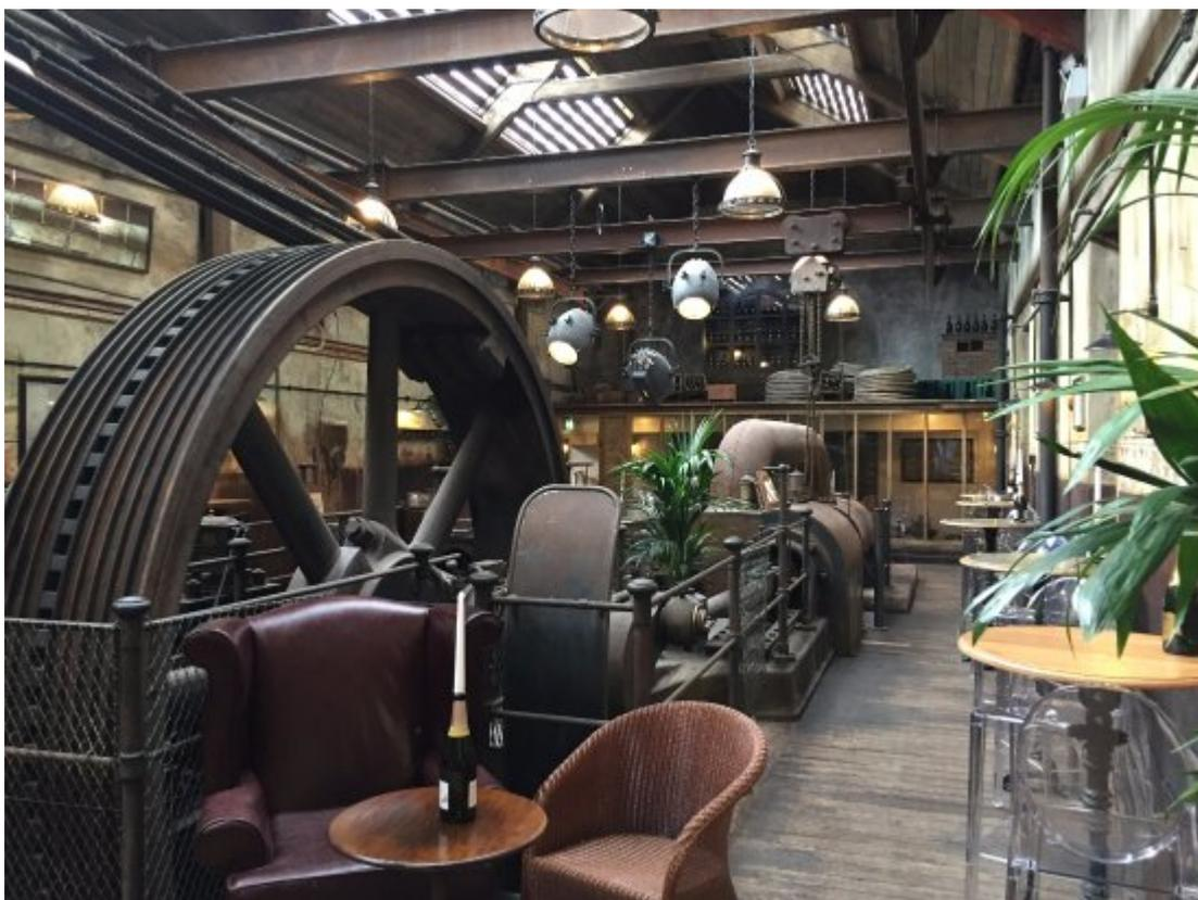
Near the centre of Clitheroe is an old mill, named Holmes Mill. It did, I believe, originally have a beam engine to power it, but later up-dated to a Clayton & Goodfellow cross-compound. Although it has not been a textile mill for many years, the engine remained in situ, although very few people managed to see it. However, fairly recently, part of the mill
